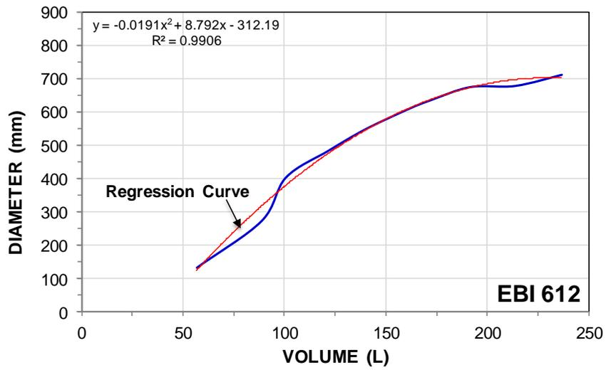
Fig. 3. EBI calibration curves – expansion in air.
